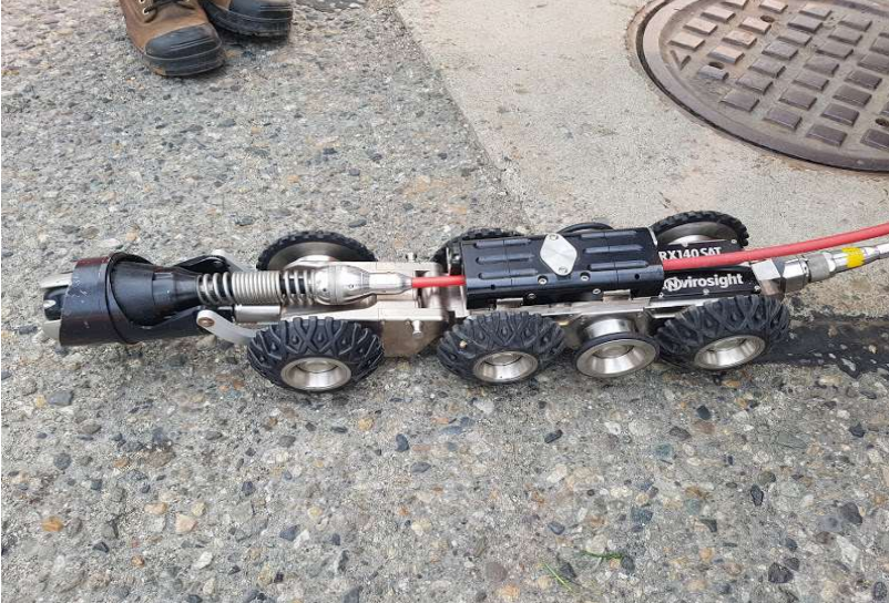
Pipe Inspection Crawler
